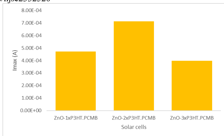
Figure 11: Maximum Current of the three samples. This figure shows the maximum currents achieved.
